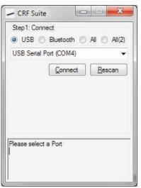
After selecting the USB radio button, CRFSuite will detect all possible options where your MSRv007 can be. They will be presented in the combo box below the radio buttons.
